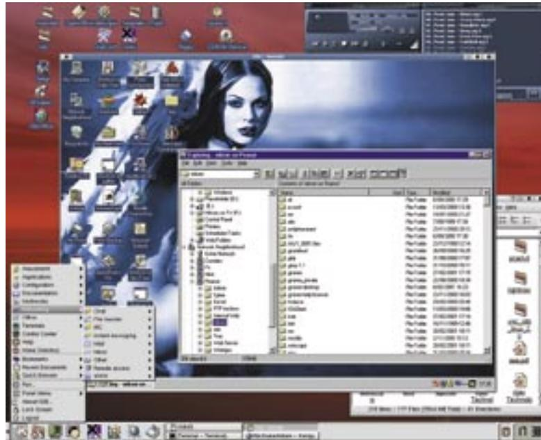
Using VNC to control a remote Windows machine from a Linux desktop.
