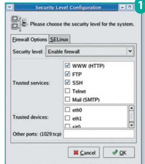
Wall of fire: The Security Level Configuration tool allows you to make rudimentary changes to the default firewall configuration.
