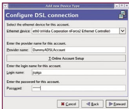
38 Setting up an ADSL modem is easy — just select the Ethernet interface that your modem is plugged in to.
